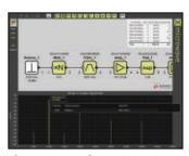
ponents (X-MWblocks) using Keysight's PNA-X analyzer. An X-parameter model of an amplifier serves as a live datasheet to determine the P1dB or IP3 at a given operating point of interest. Quickly cascade microwave components and simulate to view the spectral content at any node of the block diagram.
